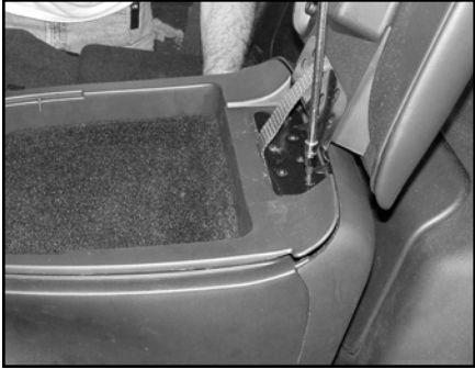
STEP 21: Mount lid strap using the "7th" T-15 Torx bolt.
